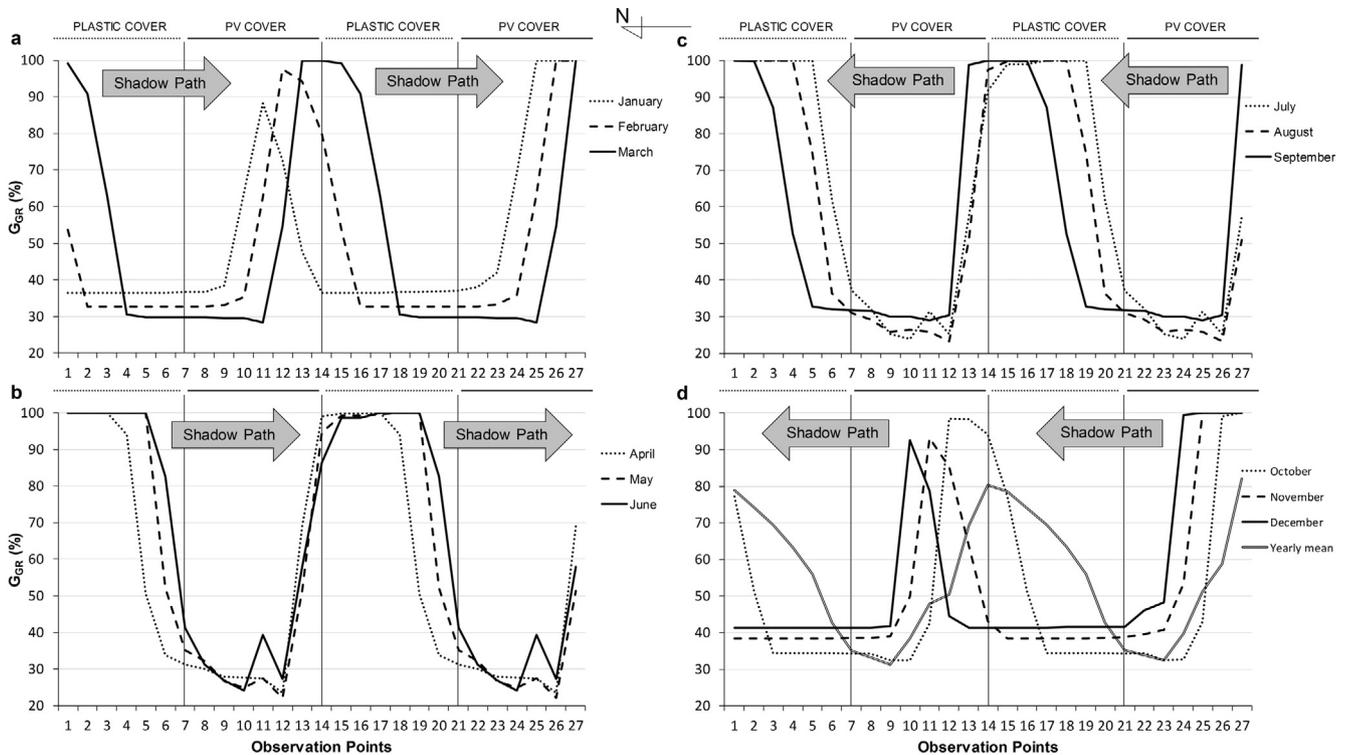
Fig. 5. Cumulated monthly distribution expressed as  $G_{CR}$  (%) on the greenhouse transversal direction (N-S) on 1.0 m height and estimated shadow path.
