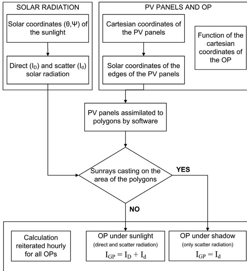
Fig. 3. Flow chart of the calculation and decisional process operated by the model via software.
