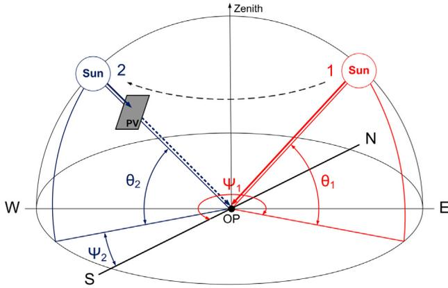
**Fig. 2.** Solar elevation angle and azimuth angle of the sun, in relation to the position of the PV panel and the observation point OP. The case 1 depicts a position of the sun in which the OP is under direct sunlight; in case 2 the OP is under the shading of the PV panel.  $\theta$  and  $\Psi$  are the solar elevation and the solar azimuth angles, respectively.
