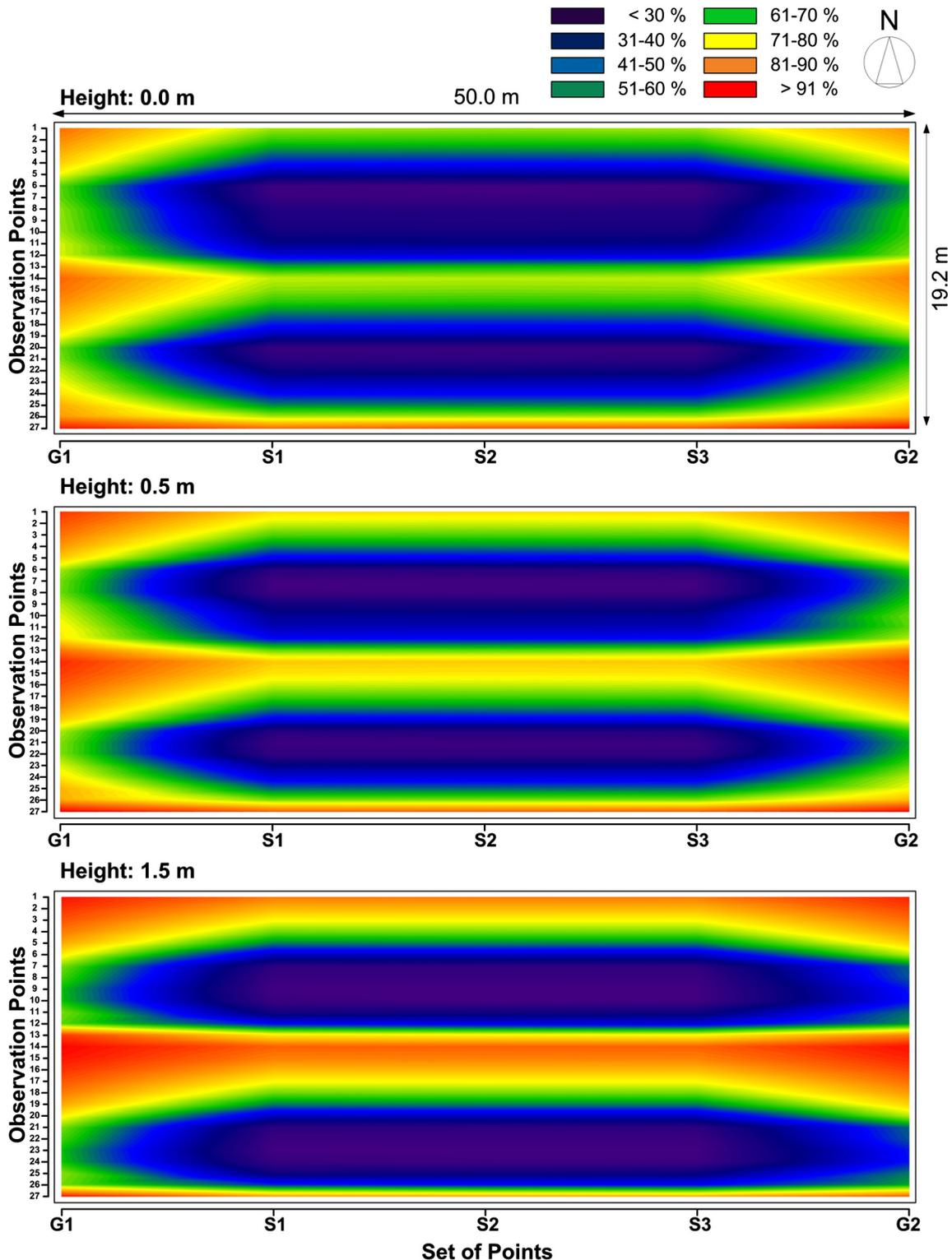
Fig. 6. Maps of the cumulated yearly light distribution on the PV greenhouse area, expressed as  $G_{GR}$  (%) on different canopy heights: ground level, 0.5 and 1.5 m.
