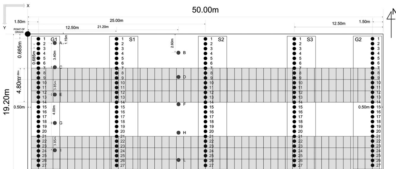
Fig. 1. Map of the PV greenhouse and position of the sets of OPs for the calculations. The OPs in grey and alphabet letters indicate the position of the pyranometers used for validating the model. The x and y axis for the Cartesian coordinates of the PV panels and the OPs are also displayed.
