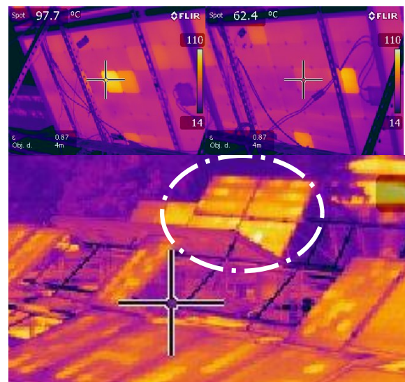
Fig. 6: Top : Two Infrared photographs of a module backsheet, with reflector augmentation taken 1 minute apart. A moving patchwork of hotspot cells is apparent. Bottom : view of multiple short-circuited modules. Only the modules highlighted with the white circle have reflector augmentation.
