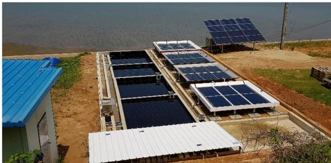
Fig. 7. Image of the salt farm parallel solar power system test bed.
