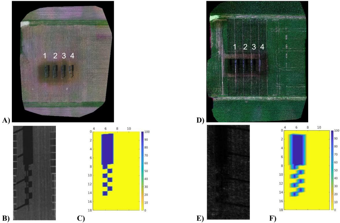
Figure 2 (a) Raw drone image taken on 6/27/19 from 3:55 PM to 4:02 PM (b) processed image of tracker 1 (c) shadow depth percentage simulation snapshot for tracker 1 (d) Raw drone image taken on 7/23/19 from 10:22 AM to 10:42 AM (e) processed image of tracker 2 (f) shadow depth percentage simulation snapshot for tracker 2.
