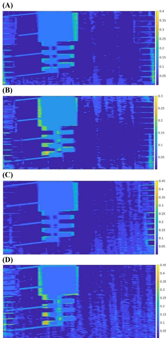
Figure 4): (a-d) contour plots of the absolute value of the difference between the drone data and the simulated snapshot for trackers T1 to T4 on 6/27/19 at 4PM
