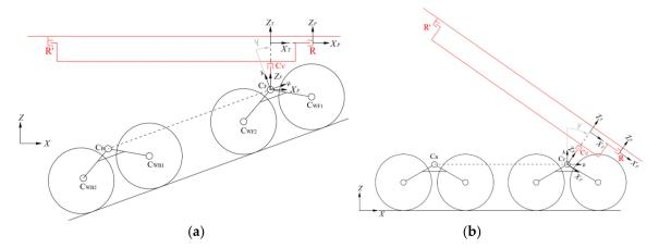
**Figure 4.** Pitch turning motions (**a**) to keep the platform horizontal above the ground; (**b**) to optimize the sunlight collection.
