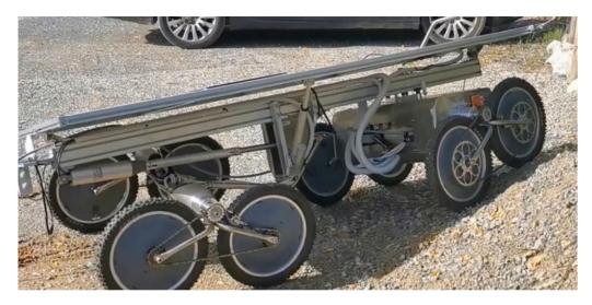
Figure 13. Agri.q02 can modify its configuration during the motion to adapt to irregular terrains.
