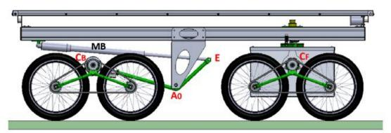
**Figure 5.** Linkage A0 - CB - E actuated by a ball screw linear actuator that permits the pitch turning motion.
