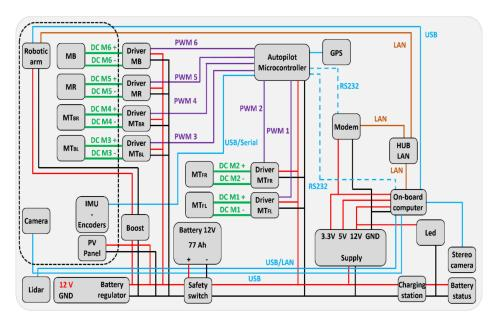
Figure 10. The mechatronic elements of the robotic system.
