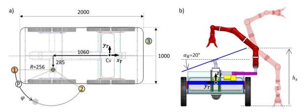
**Figure 8.** (a) The positions 1, 2, and P used to design the mobile support. Instead, 1, 2, and 3 are the three fixed mounting positions; (b) if the shoulder joint is at the height  $h_s$ , the robot can reach the terrain and still execute on-panel tasks.
