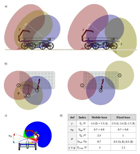
Figure 9. In (a) and (b) the mounting solution with the mobile platform is shown on the left and the one with the fixed mounting positions on the right. (a) Contribution of the pitch angle  $\gamma$  to the robot workspace augmentation; (b) platform surface covered by the robot in three different base positions; (c) variation of the workspace due to the motion associated to the roll angle  $\alpha_R$ ; (d) summary table with the values of the indices with mobile and fixed base.
