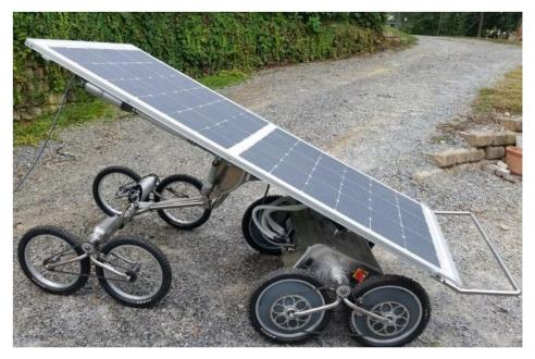
Figure 12. The prototype of Agri.q02 in the sunlight collection configuration.
