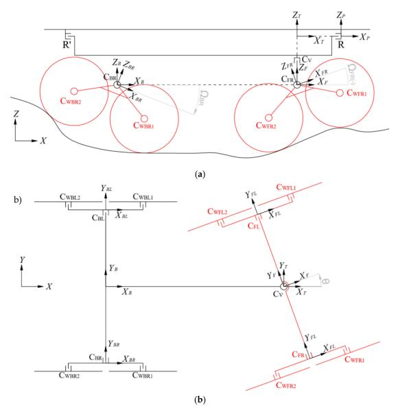
**Figure 3.** (a) Rotations of the rocker arms that permit to keep the wheels in contact with the ground even in the presence of irregularities of the terrain; (b) controlling the rotational speed of the two motors  $MT_{FR}$  and  $MT_{FL}$  it is possible to rotate the front box with respect to the back chassis in order to obtain the desired trajectory for the rover.
