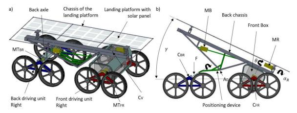
Figure 2. (a) Agri.q02 functional design; (b) functional design with the ten modules.
