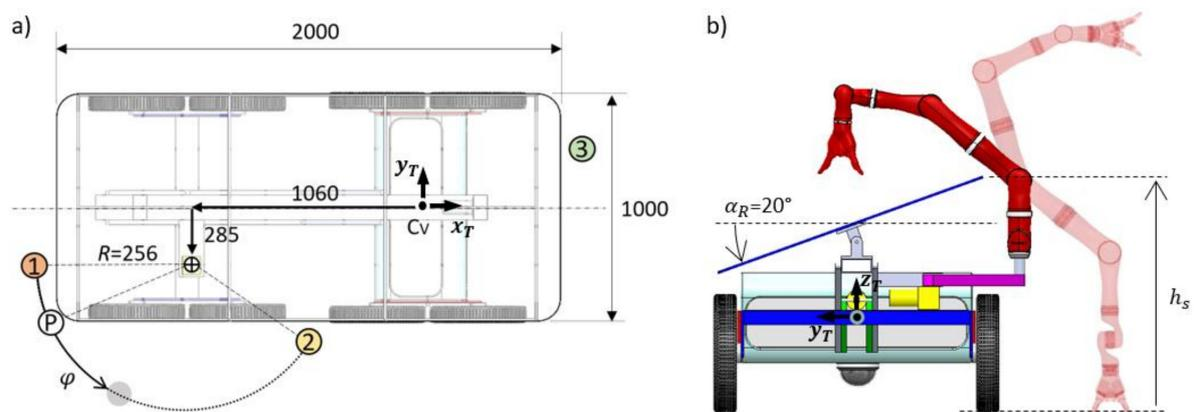
**Figure 8.** (a) The positions 1, 2, and P used to design the mobile support. Instead, 1, 2, and 3 are the three fixed mounting positions; (b) if the shoulder joint is at the height  $h_s$ , the robot can reach the terrain and still execute on-panel tasks.
