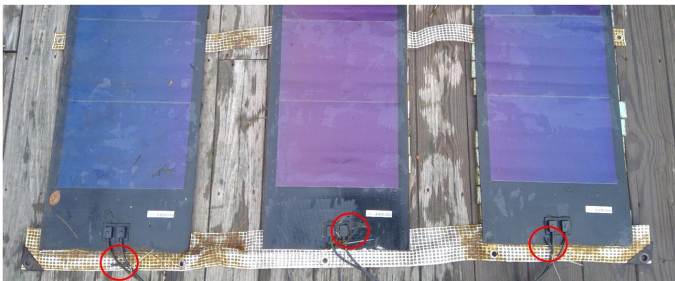
*Figure 6. Top surface of FPV array after three months of deployment in the Portage waterway with temperature sensors circled in red.*
