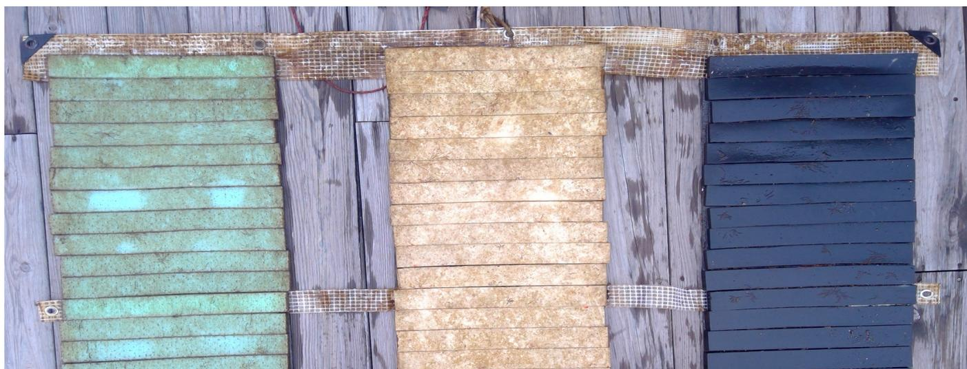
*Figure 7. Algal accumulation after deployment on the underside of the foam. Foam types left to right: PE, Mincel T, neoprene.*
