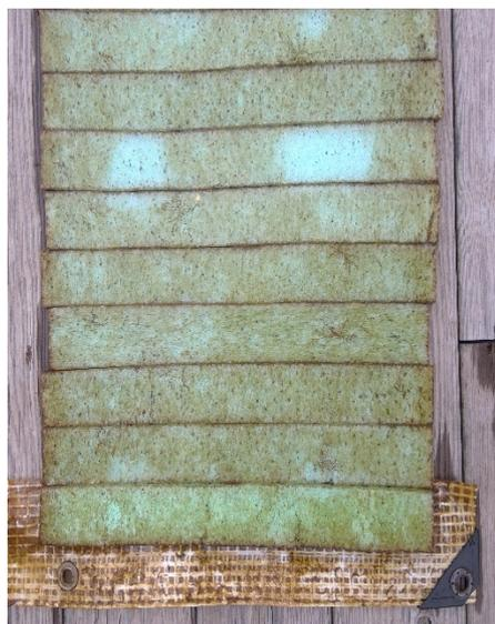
*Figure 8. Details of algal growth for a) PE shows surface and internal algal accumulation b) Mincel T shows surface accumulation c) neoprene shows solids stuck to the surface*
