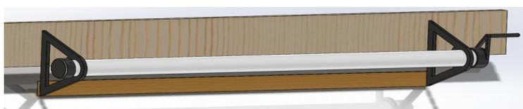
Figure 2. a) CAD design of FPV deployment system and basic mooring design b) side view and c) top view.
