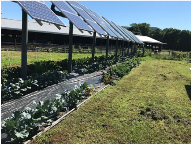
Figure 2.1: The AV Photovoltaic Dual-Use Research Project set-up at the UMass Crop Research Farm in South Deerfield, Massachusetts.
