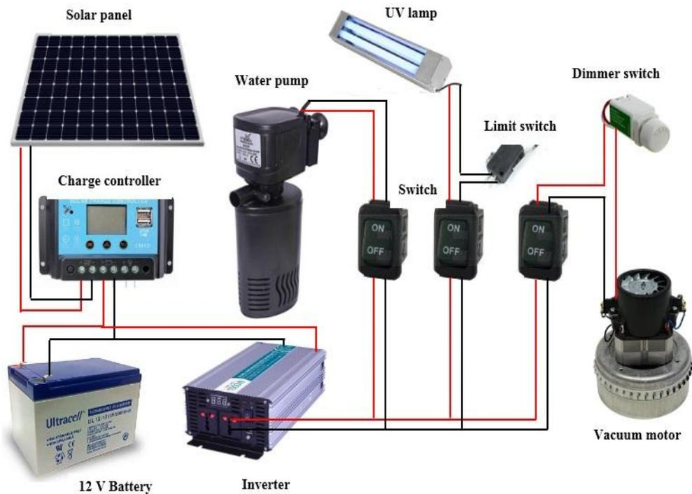
**Fig. 8:** The electric circuit of the whole managing unit
