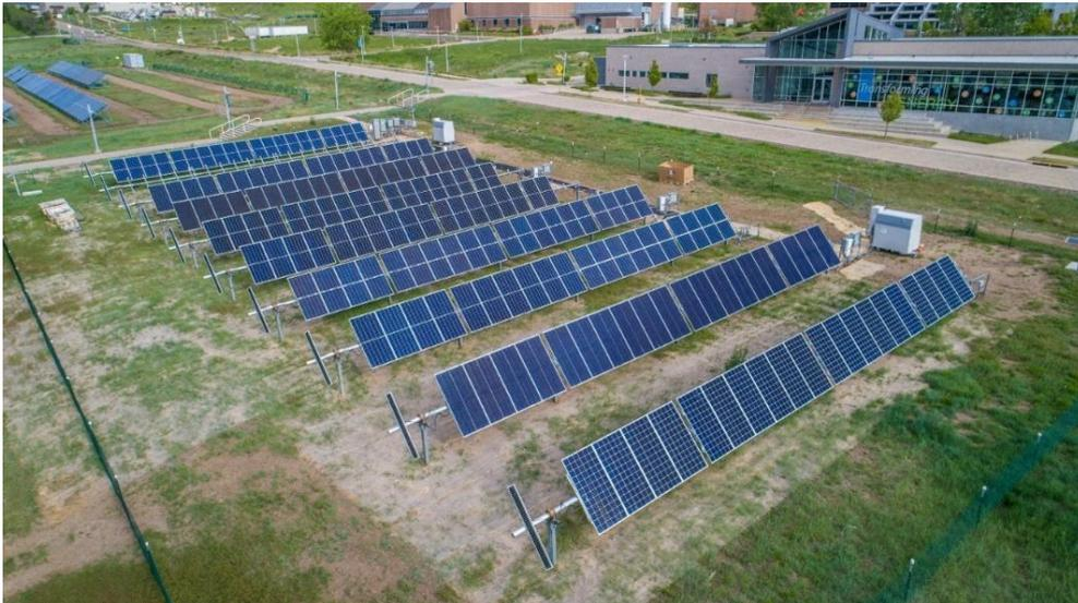
Figure 15 Picture of the bifacial PV modules installed at NREL BEST-field (Ayala & Deline, 2020b). Reprinted with permission.
