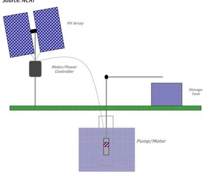
The size and number of panels is determined by the voltage requirements of the pump. The size and type of pump, in turn, is determined by the amount of water needed and the height and distance the water needs to be pumped.
