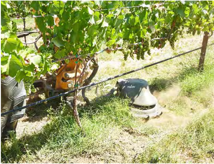
An in-row vineyard weeder removes weeds at the soil surface without exposing soil to tillage. Photo: Rex Dufour, NCAT
