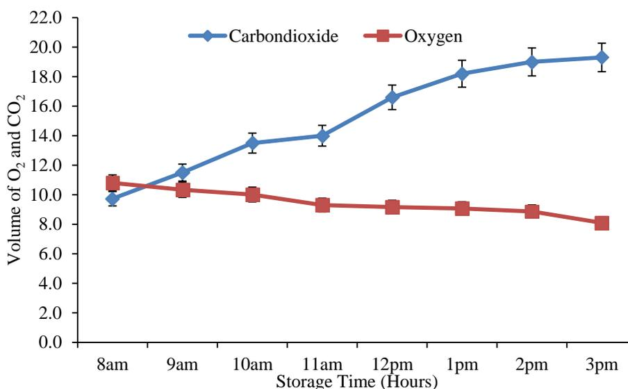
**Figure 5.** Changes in CO<sub>2</sub> and O<sub>2</sub> concentrations (ppm) with time within the conventional cooling chambers.
