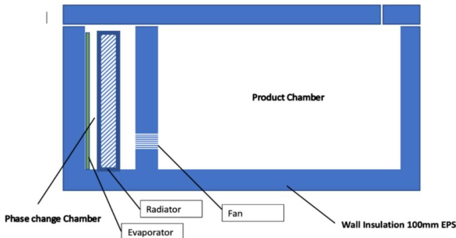
Figure 1. Schematic diagram of the solar cooler.
