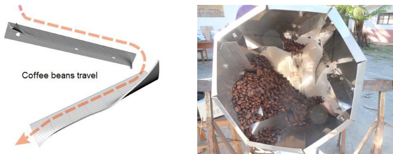
Figure 5: Final design of blades in the medium size drum to ensure homogeneity of coffee roasting
