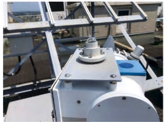
Fig. 10. Pyranometer used for global total irradiance measurement.
