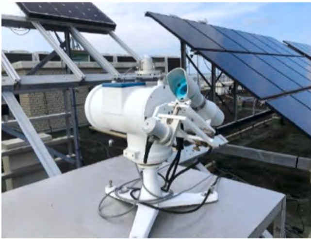
Fig. 11. Pyrheliometer with a 2-axis tracker for measurement of direct normal irradiance.
