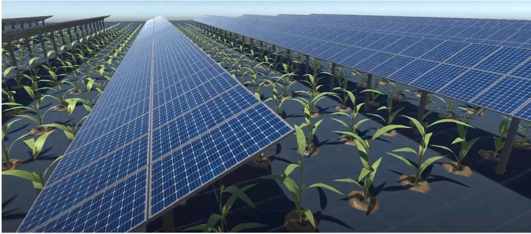
Fig. 1. Field style agrivoltaic system designed in Unity3D.
