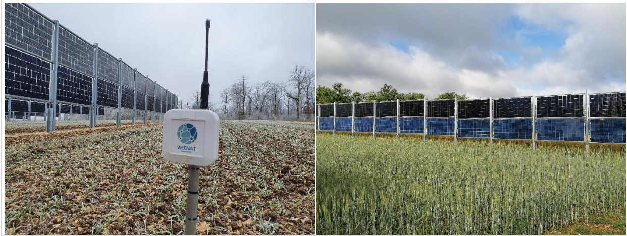
Figure 8. Agrivoltaic system of TotalEnergies at Channay in central France (left picture shows tensiometers that are used and right picture shows wheat growing in the system)
