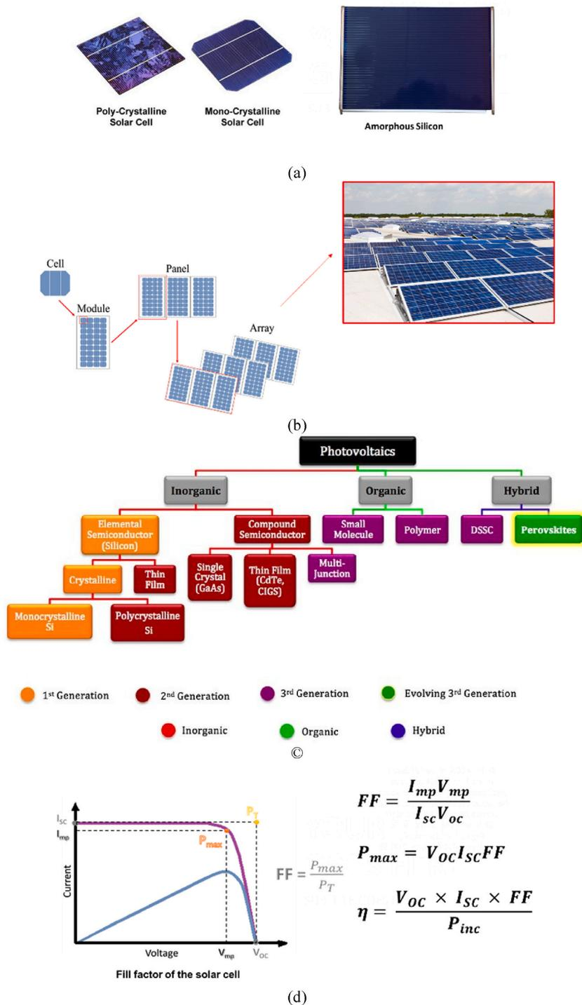
Fig. 2. (a) solar cell, (b) photovoltaic module, (c) PV classification, (d) I-V characteristics.
