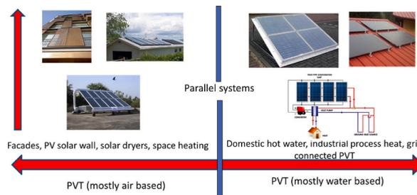
Fig. 5. Integration of PV-T system applications.
