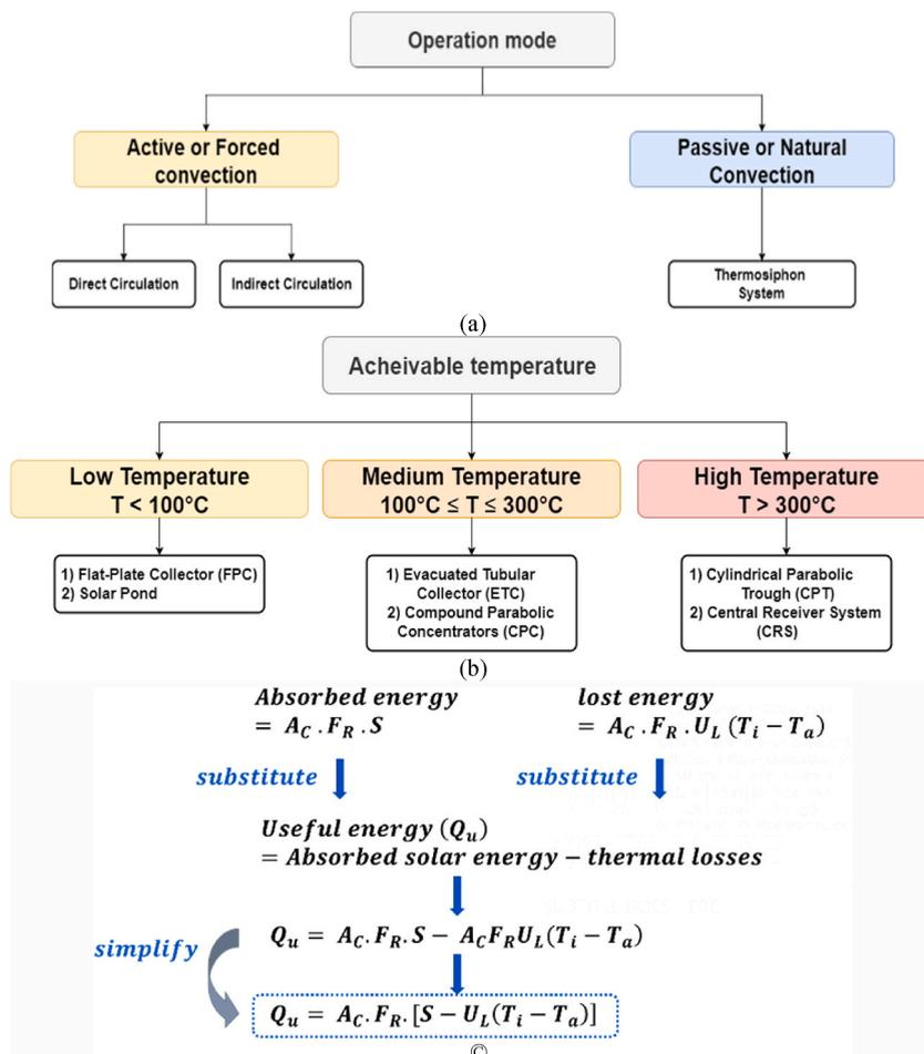
Fig. 3. Solar thermal collector classification based on (a) operation mode, (b) achieved temperature, and (c) energy calculations.
