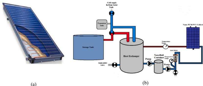
Fig. 1. PV-T (a) collector, (b) system [34].
